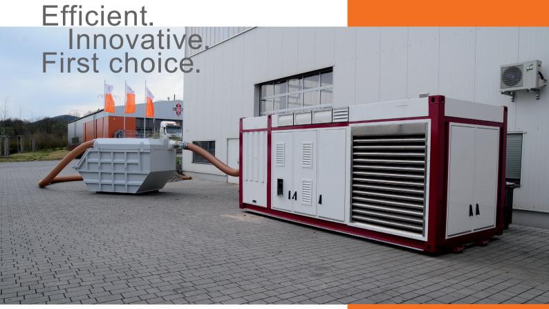
With the Container-Suction-Unit (CSU) RSP provides a flexible stationary solution for a whole range of applications. The CSU could either be worked stationary or mounted onto a vehicle, a trailer or a railway carriage. It consists of a suction-unit and a separate material-container with a capacity of up to 8 cbm. A choice of connection- and extension hoses is completing the system.
